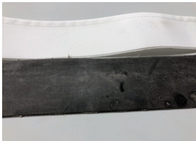
Newer dacron sailcloth CB gasket top of picture. Older rubber one below.
