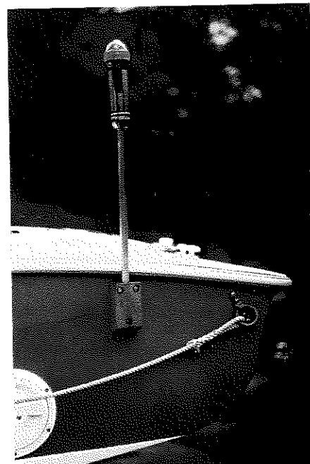
The all-round light in its mounting block on the transom. This is an older model; the current Fulton lights have a larger and quite different lens.
