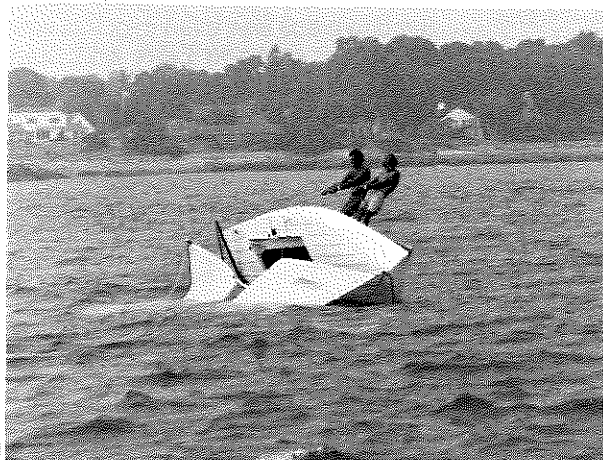
With weight fully extended, the balance shifts and the boat starts to come up. Note that the 'back-winded' jib, holding many gallons of water, is acting somewhat as a brake, hurting the boat's righting.
