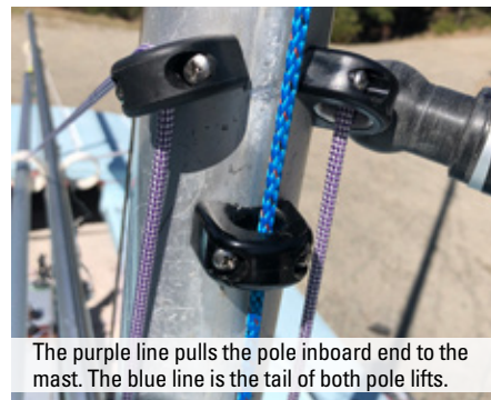
The spinnaker sheets pass through rings. The downhauls pulls the rings tight to the pole ends.
