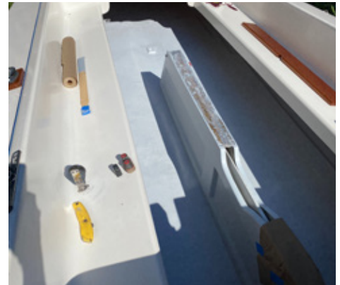
Fresh gel-coat with non-skid.
