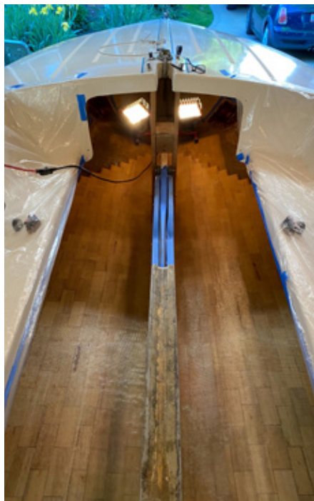
New balsa glassed in, ready for gel-coat.
