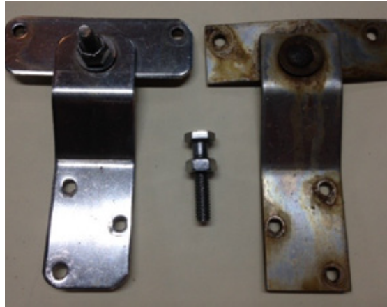
Forestay toggle plates: old one with rusted rivet on right, newer plate with pivot bolt on left.
