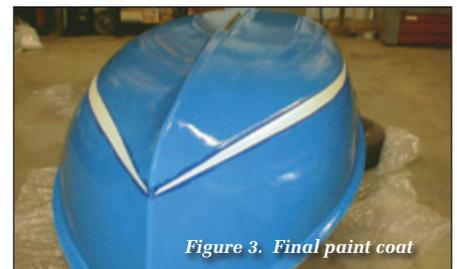
Figure 3. Final paint coat
