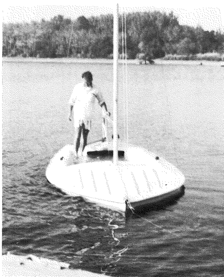
Builder swamped a Flying Scot to show how the boat floats filled with water.
